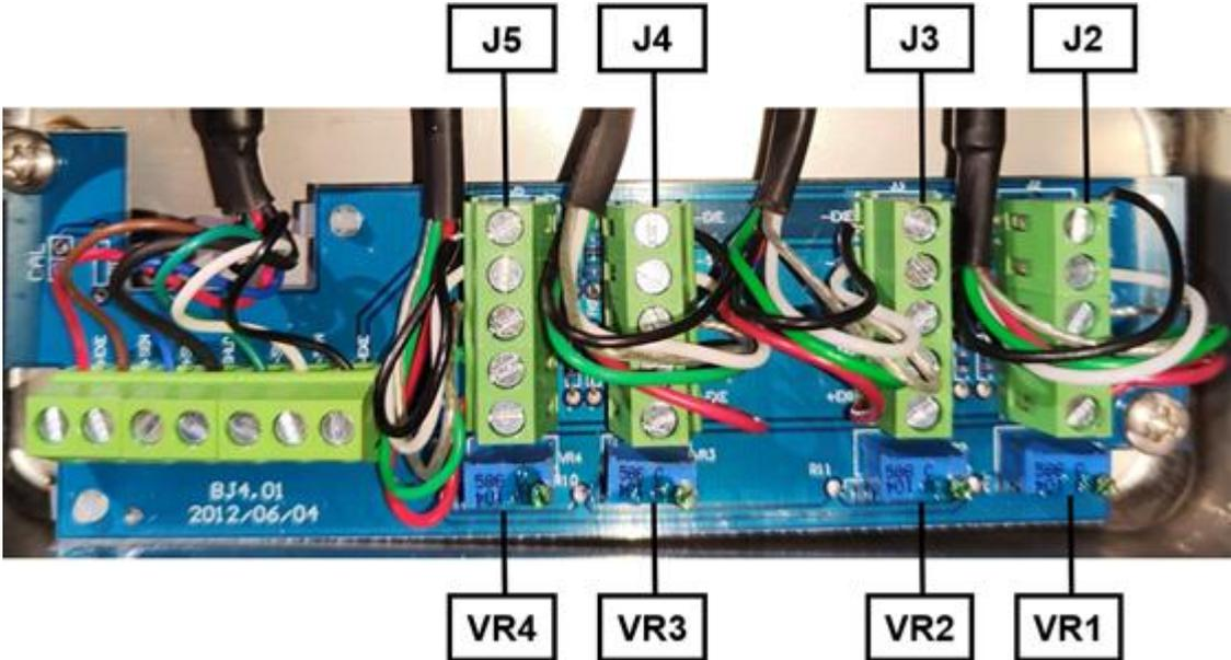
The load cell J2 is adjusted using potentiometer VR1.
