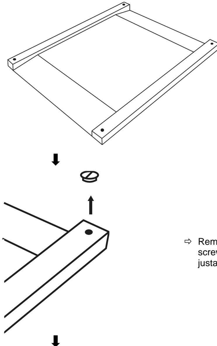
⇒ Remove the cover screws from the adjustable feet (4x)
