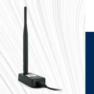
MadgeTech's RFC1000 is a powerful wireless transceiver for use with RFOT and 2000A series data loggers. The RFC1000 transmits to other RFC1000s up to 4000 feet outdoors/line of sight, 1000 feet typical indoors/urban. The RFC1000 transmits to data loggers up to 2000 feet outdoors/line of sight, 500 feet typical indoors/urban. Additional RFC1000s can be used as repeaters to transmit greater distances or around obstacles.
