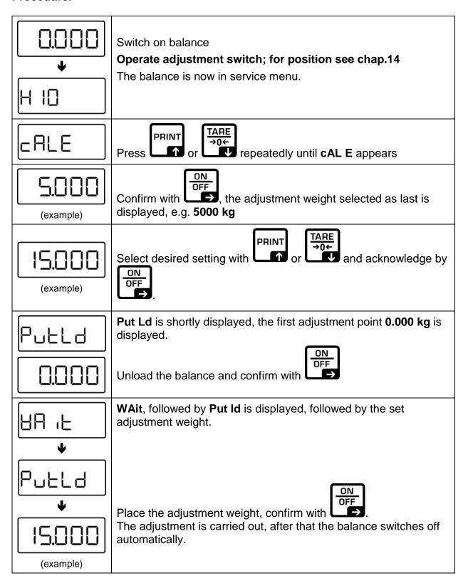
An adjusting error or incorrect adjustment weight will generate an error message ("Err 4"), repeat the adjustment process.
