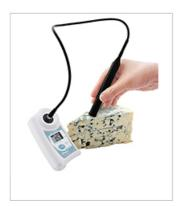
The PAL-SALT PROBE features convenient operation of submerging the probe in a liquid for measuring the salt content in as fast as 3 seconds. The probe may be inserted directly into semi-solid food. However, measurements at different locations may be inconsistent, and such direct measurements may vary from measurements by dilution methods.
