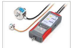
Simultaneous measurement on up to four channels. External sensors with sensor data memory, optionally available, see *Measuring Cells*
