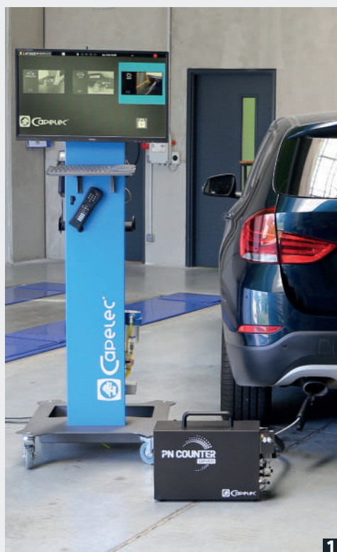
1 Gas + Particle analyzer + touch-screen PC on Totem (optional mobile holder)
