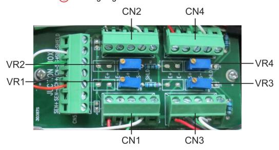
Adjustment of weighing cell CN1 takes place at potentiometer pair VR1. Adjustment of weighing cell CN2 takes place at potentiometer pair VR2. Adjustment of weighing cell CN3 takes place at potentiometer pair VR3. Adjustment of weighing cell CN4 takes place at potentiometer pair VR4. Increase the value turning to the right, reduce the value turning to the left.
