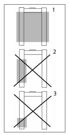
The U-weighing bridge is designed for an even distributed load
