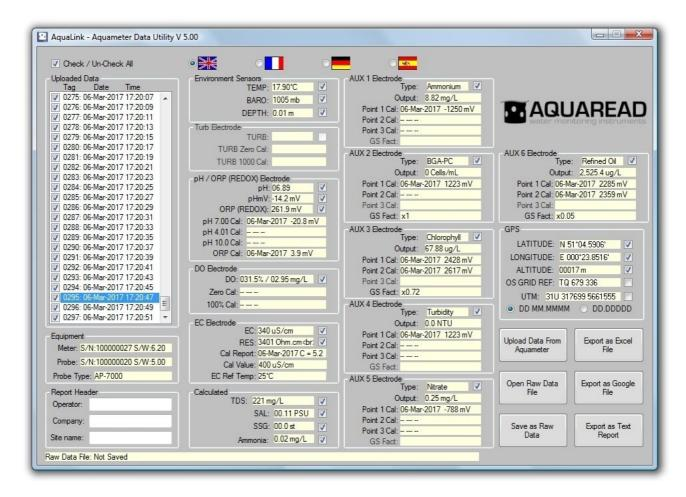
To view any of the logged data records, simply click on the desired Tag, date and time label as shown above. The data for the highlighted label will be displayed in the individual data boxes, which are grouped by electrode function. Any data that is unavailable or out of range will be displayed as dashes. To move up and down the Tag/date/time column, use either your mouse or the cursor up/down keys.
