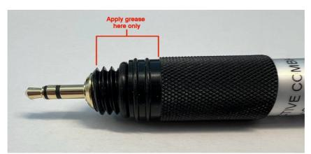
Using a clean cloth or tissue paper, polish the gold contacts ensuring they are completely clean. Carefully insert the electrode into the AUX socket and tighten firmly until the O-ring is completely compressed.
