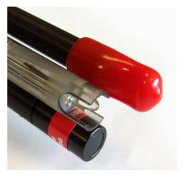
The caps should be fitted to all ISE Electrodes when using pH calibration solutions or other ISE calibration solutions other than that specific for the ISE being calibrated in order to protect the ISE electrodes from the effects of the buffer solution and interfering ions.
