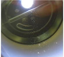
If your zero calibration water is aerated, allow it to stand for a while until the air has all dispersed, then re-insert the Probe and re-calibrate. Do not leave the Probe sitting in aerated water, the bubbles will simply cling to the inside surface of the Probe and make the problem worse.
