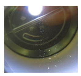
If your zero calibration water is aerated, allow it to stand for a while until the air has all dispersed, then re-insert the Probe and re-calibrate.
