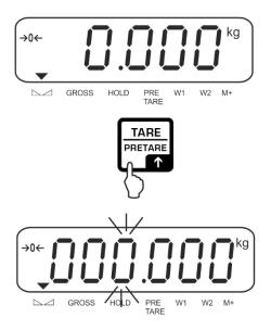
⇒ Enter known tare weight (e.g. 2 kg) by operating the navigation keys and confirm by pressing the zero key. Numerical input, see chap. 3.1.
