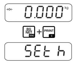
The screen <SET h> used to enter the upper limit will be displayed. Press the ZERO key, the current setting appears.
