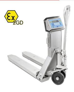
AISI 304 stainless steel pallet truck scale for use in ATEX hazardous areas 1 & 21 & 2 & 22, with Ex II 2G IIB T4 Gb X and Ex II 2D IIIC T197°C Db X protection modes. Available in approved version for legal-for-trade use. Manufactured, calibrated and adjusted in Italy by Dini Argeo, using certified sample masses.
