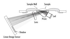
In the **HI 96831** refractometer, light from an LED passes through a prism in contact with the sample. An image sensor determines the critical angle at which the light is no longer refracted through the sample. Specialized algorithms then apply temperature compensation to the measurement and convert the refractive index to: % Volume or Freezing Point.
