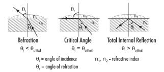
The critical angle can be used to easily calculate the refractive index according to the equation:
