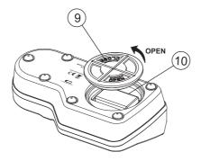
9. Battery Cover10.Battery Compartment
