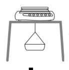
⇒ Attach empty immersion basket to the hook for underfloor weighing.
