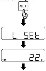
⇒ When the balance is in the measuring mode, hold down the [SET] key for about 2 seconds.
