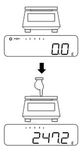
⇒ You can check whether the weight value shown on the display changes using light finger pressure on the weighing plate,
