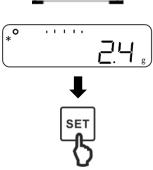
⇒ Place the first sample on the weighing plate and wait until the display shows an asterisk <\*>.
