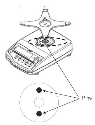
2. Place the weighing plate on the weighing plate carrier
