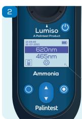
The wavelengths of light the instrument uses are shown in nanometres (nm).
