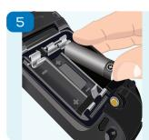
Insert new batteries in the same way, pushing towards the negative contact, but this time, down at the positive end.
