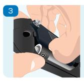
The cover will lift and, if necessary, the captive screw can be further loosened so the cover can be removed completely.
