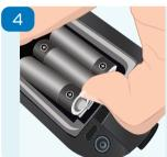
The batteries are held firmly in place by the clips to enhance Lumiso's resilience to physical shock.
