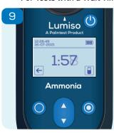
For tests with a "wait time" (see test instructions), a preset timer will count down and then automatically commence reading.
