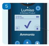
The instrument will measure the blank and show when this has been successful.
