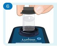
Ensure that your Lumiso Instrument is clean and dry. Place photometer tubes in the instrument with white diamond aligned to the mark on the instrument.
