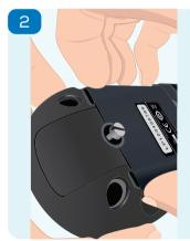
The watertight seal built into the battery cover means that a firm pulling force needs to be applied to remove it.
