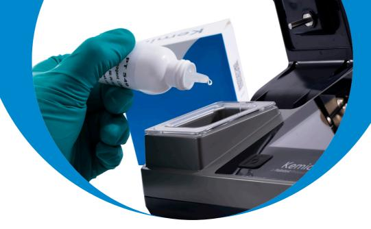
**Testing for** Bromine, Chlorine, Chlorine Dioxide, Chlorite and Peracetic Acid
