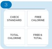
Press the back button to return to the CONFIGURATION menu. It is not possible to navigate away from the screen without at least one test type selected.
