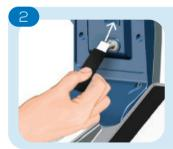
Open the arm, and insert the first of three check standards from the KEMC10 pack.
