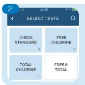
Highlight test types by pressing them. A number appears in the bottom right corner. The number represents the order in which they appear on test selection screens.
