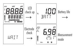
Note: The meter detects the presence and the type of the probe at its input.
