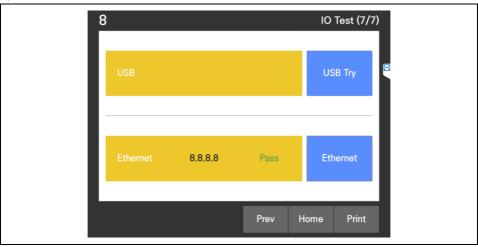
4) Once the tests are complete, press "Print" button to print the results.
