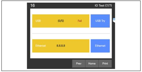
3) Click "Ethernet" button to test Ethernet communications.
