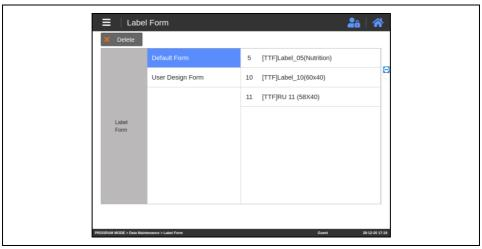
3) 'User Design Form' is a label form saved by the user in the scale, and can be deleted by clicking the 'Delete' button after checking the check box.
