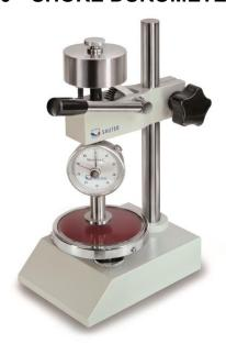
The test stand TI for Shore hardness testers can be purchased in addition, optionally to the HB hardness tester.
