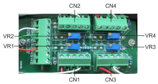
Adjustment of weighing cell CN1 takes place at the potentiometer VR1 Adjustment of weighing cell CN2 takes place at the potentiometer VR2 Adjustment of weighing cell CN3 takes place at the potentiometer VR3 Adjustment of weighing cell CN4 takes place at the potentiometer VR4 Increase the value turning to the right, reduce the value turning to the left.
