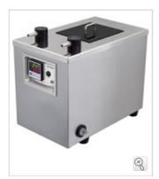
The 60-C5 is an external circulation type constant temperature water tank provided with a thermomodule. The temperature can be set in the range of 10 to  $60^{\circ}$ C and the unit is perfectly suited for connection with a refractometer. An upgraded version of the 60-C4 model, featuring an increased tank capacity of 1.0L and an improved resolution of  $0.1^{\circ}$ C which makes it even easier to use.
