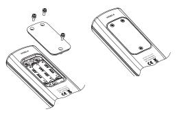
Replace the three 1.5V AAA alkaline batteries located in the battery compartment, observing the indicated polarity.
