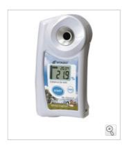
This model can be used for determining the quality of colostrum to protect and nurture the health of your livestock and newborn calves! The ideal colostrum (first milk) Brix level is 20% and above.It measures the Brix value of colostrum, which has a correlation with the immunoglobulin (IgG) value contained in colostrum. If the Brix value of the colostrum is over 20%, you can safely assume it is high-quality colostrum.
