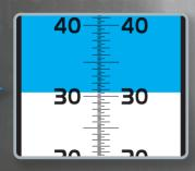
**3** Read the measurement value where the boundary line intersects the scale.
