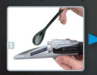
Apply 1-2 drops onto the prism.
