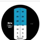
This model has an automatic temperature compensation function.
