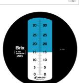
Can be widely used for beverages, fruit juices, soups, beef bowl sauce, water-soluble cutting oil, etc. MASTER-M is made of metal, and MASTER-PM is plastic. For salty and acidic samples, choose the plastic body, MASTER-PM. This product is the cheapest type with no temperature compensation function. Since the concentration changes as the measurement temperature changes, MASTER- $\alpha$  and MASTER-T are recommended if you have trouble managing the temperature at each measurement.
