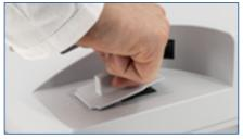
Fig. 4: Remove cuvette slot cover
