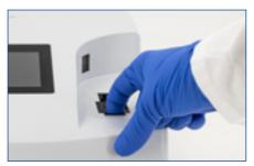
Fig. 5: Remove cuvette adapter
