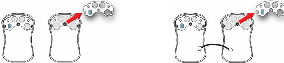
5. Grip the currently installed waterproof membrane filter and pull it up. You may have to use a tweezers to get a firm grip. (If it leaves residue, blow it out with a can of compressed air.) Discard the used waterproof membrane filter.
