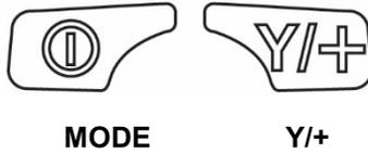
In addition to their labeled functions, the keys labeled [MODE] and [Y/+] act as “soft keys” that control different parameters and make different selections within the instrument’s menus. From menu to menu, each key controls a different parameter or makes a different selection.
