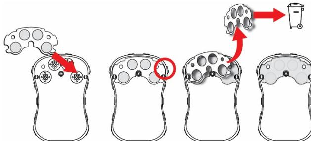
10. Inspect the rubber seal (PN: M03-2004-000), and if it is damaged or cracked, replace it.
