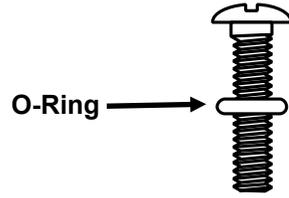
To prevent damage to the housing, the screw, and the O-ring, an electric screwdriver should be set with torque less than 3kgf.cm, and a speed rate of less than 670r/min.
