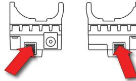
Align the Travel Charger with the middle of the MicroRAE, squeeze the latches on both sides of the Travel charger, and press it until it is firmly attached to the MicroRAE. Then release the latches. Make sure you press the latches close to the instrument instead of at their ends.
