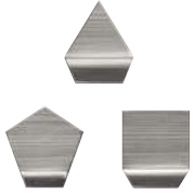
Milligram weights, flat polygonal sheet
