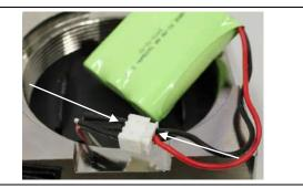
Insert battery in the centre. Ensure that the cables are not kinked. Relock battery compartment.
