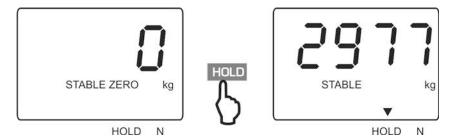
⇒ The peak load will be held on the display until deleted by pressing **HOLD**-key.
