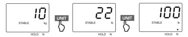
Every time the **UNIT**-key is pressed, the next weighing unit will be displayed.  $kg \rightarrow lb \rightarrow N$ .
