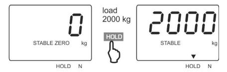
⇒ The weighing value will be held in the display until it is deleted by **HOLD**-key.
