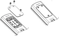
Replace the three 1.5V AAA alkaline batteries located in the battery compartment, observing the indicated polarity.
