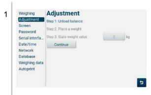
Unload the balance. Ensure that there are no objects on the weighing pan. Tap <Continue>.
