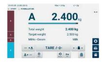
Weight of the component is below the desired weight/tolerance
