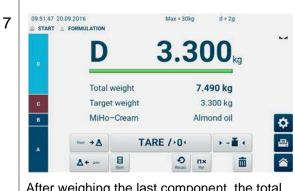
After weighing the last component, the total weight and individual weights of the components can be printed out by connecting an optional printer (depending on the setting in the menu either automatically or after
