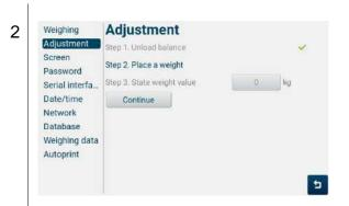
Place the adjustment weight at the centre of the weighing pan. Tap <Continue>.
