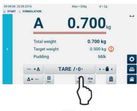
If a nominal weight is exceeded, press and the nominal weights of the other components are calculated proportionally to the exceeded weight value.
