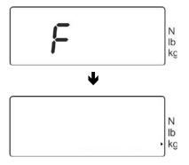
After adjustment the balance turns itself off again automatically. In case of an adjustment error or wrong adjustment weight "E" is displayed, repeat the adjustment process
