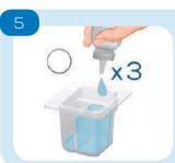
If chlorine or copper is present in the solution, add 3 drops of Glycine reagent to prevent them from interfering with the measurement. Use the stir rod to mix the sample. If no chlorine or copper are present, skip this step.
