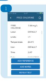
The first line displays the test type and the measured concentration (after dilution if applicable).
