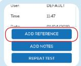
Press ADD REFERENCE to add information from a barcode (or the information can be typed in manually) to enrich the data record. See p. 9 in the instruction manual for details on producing and using barcodes.
