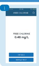
At the end of the countdown, the test results will display on screen. The number of results displayed depends on the test type.
