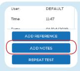
Press ADD NOTES to type information about the test using the on-screen keyboard. Maximum of 48 characters. After a failed test, it is recommended to write an explanatory note or explain the corrective actions taken, as the information will be stored alongside the test in memory.
