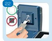
Hold the final CDX sensor through the foil packet only, with the white side facing up. Slide it all the way in, until the end stops against the back of the slot.
