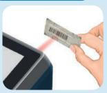
Scan the sensor barcode using the barcode scanner when prompted. Hold the barcode about 10cm (4in) from the instrument. Align the red dot with the center of the barcode. When the scan is complete, the instrument proceeds to the next screen.
