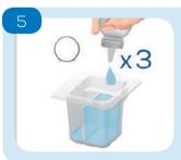
If chlorine or copper is present in the solution, add 3 drops of Glycine reagent to prevent them from interfering with the measurement. Use the stir rod to mix the sample. If no chlorine or copper are present, skip this step.
