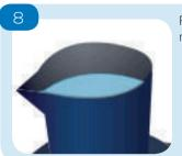
Fill the degasser vessel up to the mark with fresh sample.
