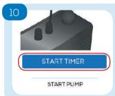
Press the START TIMER button to begin the timer. The displayed time is calculated based on the concentration of chlorine dioxide measured in the previous step.
