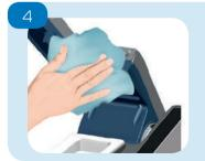
If Kemio is wet, wipe it down with a cloth according to the care and maintenance suggestions. Take special care of the electrical contacts. These can be accessed by opening the front lid of the arm.
