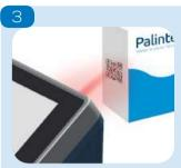
Scan the QR code on the side of the box of sensors. Details about the batch appear in a pop up on screen, and is automatically sorted into the correct folder. If a batch is added as a duplicate, the "loaded on" date will update but nothing else will change.
