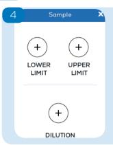
Add a lower limit and/or upper limit to set the range that is considered a PASS for the test application.
