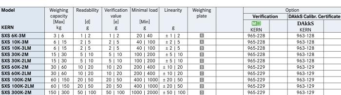
Dual-range balance switches automatically to the next largest weighing capacity [Max] and readibility [d] Note: For applications that require verification, please order verification at the same time, initial verification at a later date is not possible. Verification at the factory, we need to know the full address of the location of use.
