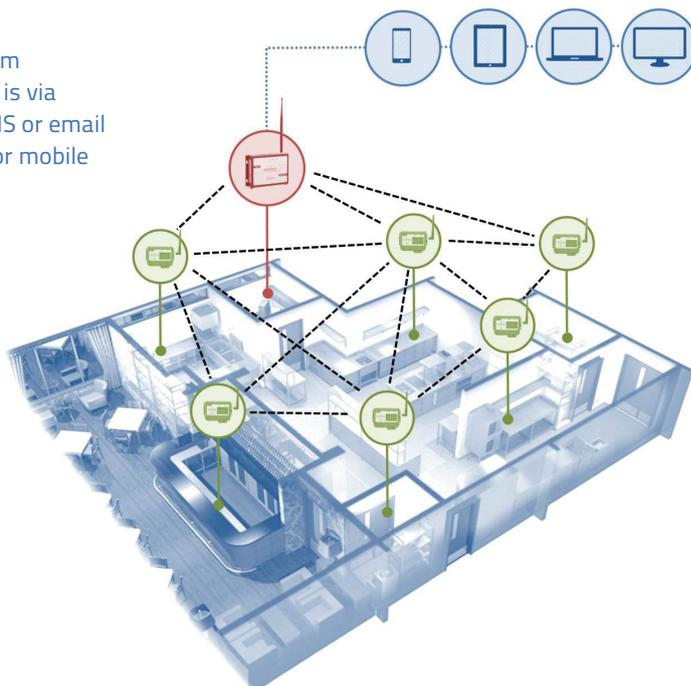
The above schematic shows an example of RF500 mesh network. In the event of signals being blocked to or from a specific route, RF500 Transmitters automatically seek an alternative route across the mesh network.
