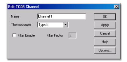
9. From the **Thermocouple** drop-down list, select the type of thermocouple you are using and click **OK.**
