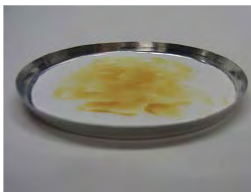
Water and oils evaporate, minor discoloration
