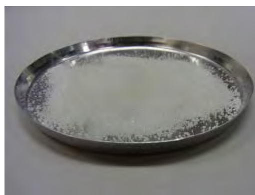
No discoloration, but surface slightly solidified.
