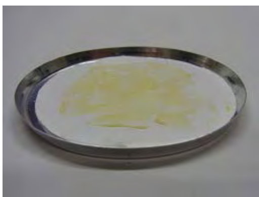
Sample distributed evenly by a spatula at a fiber glass filter
