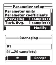
**Note** Each reading takes 1 second, so when logging the first sample will be delayed by a few seconds if averaging is used.
