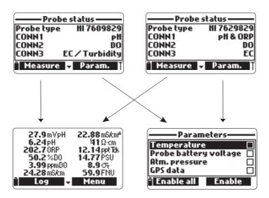
The probe status screen identifies the probe and attached sensors. Non-logging probes are identified as HI 7609829 and logging probes are identified as HI 7629829
