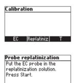
Put the probe into a beaker with replatinization solution and press Start.
